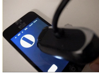
Fig. 12. Data input by rotating finger to turn the visual knob on the screen
