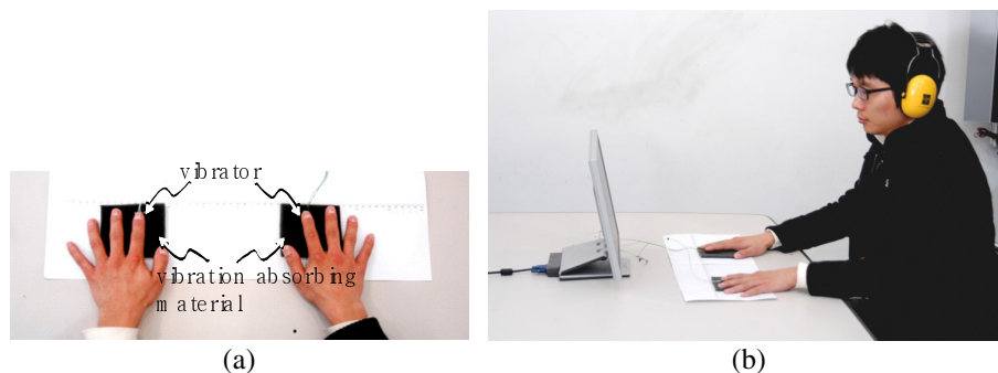
Fig. 1. (a) Stimulation of vibrotactile feedback on both hands (b) Presentation of vibrotactile feedback through the vibrator
