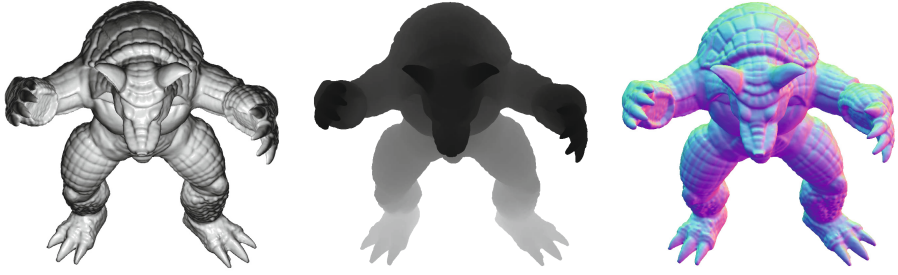
Fig. 1. Comparison of a generated depth map (center) and normal map (right) of a particular viewpoint of the armadillo model (left). High frequency details cannot be stored in the depth map due to limited spatial resolution. In contrast, high frequency details are better preserved in the normal map.
