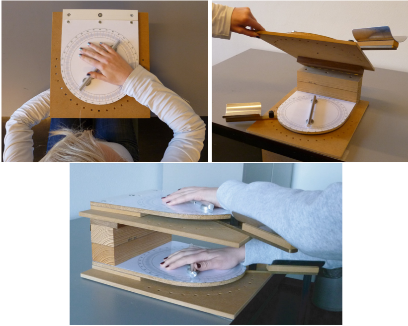
Fig. 2. Set-up used in the experiment. Top left: top view. The arm angle of the participant is 120^\circ . Top right: the upper plate could be unfolded to get easy access to the lower plate. Bottom: side view. The arm angle of the participant is 60^\circ . Notice in the top right and bottom pictures the arm rests, that could be adjusted in order to fix the orientation of the arms of the participant.
