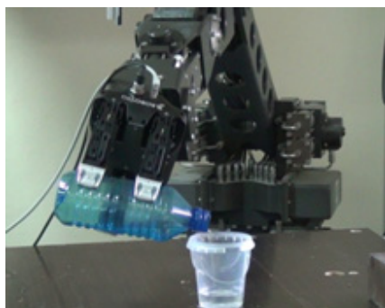
Fig. 8. 3-Finger hand Robotiq connected to a Kraft Grips manipulator. Future application will focus on using the developed device to control this system.
