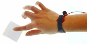
Fig. 4. Remote tactile feedback provided by wrist-worn actuators during tabletop interactions
