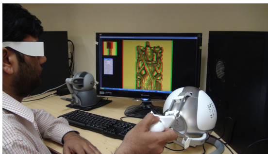
Fig. 9. Illustration of haptic-visual immersion of a subject for a virtual cultural heritage object. On the right, the user wearing anaglyphic glasses is holding the FALCON haptic device while interacting with the cultural heritage model displayed on the screen.
