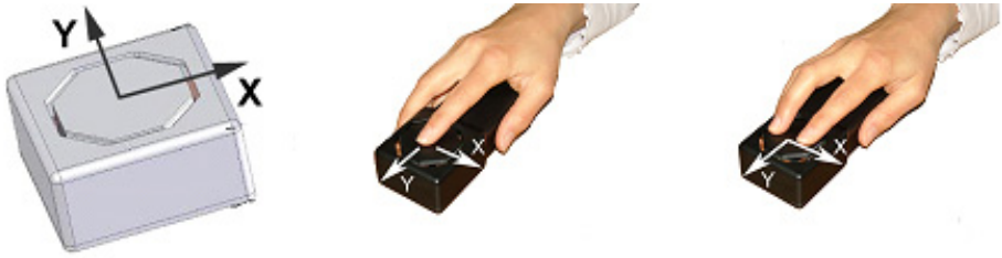
Fig. 1. The Viflex device with its octagonal platform (left). The device with its battery extension handle can be used with one (middle) or two (right) fingers.
