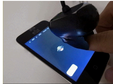
Fig. 13. Data input by changing contact angles of the finger at arbitrary positions on the screen
