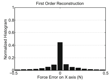
(b) Force error when using a first-order PD compression.
